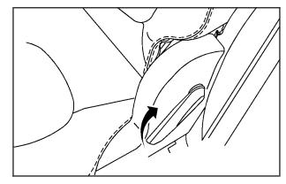
Pull up on and hold the lever located on the side of either rear seat. Notice: Folding a rear seat with the safety belts still fastened may cause damage to the seat or the safety belts. Always unbuckle the safety belts and return them to their normal stowed position before folding a rear seat.
